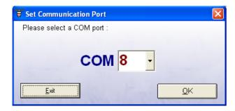
On starting the virtual front panel for the first time, a COM port selection screen will be displayed. Click on the COM port which is connected to your 3000 Series calibrator to continue.
